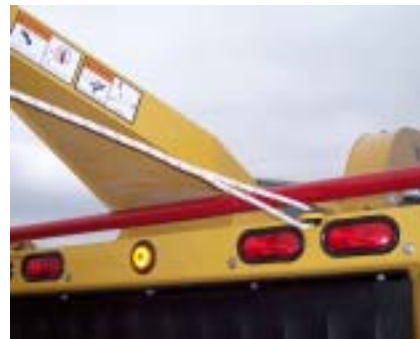
Winch line Safety Interlock and Storage Hook
